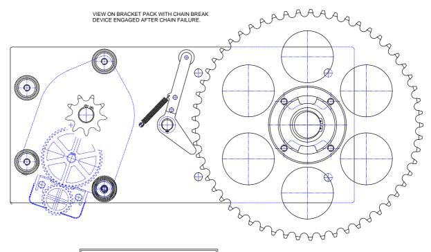
THIS IS A CHAIN BREAK DEVICE IT DOES NOT PROTECT AGAINST SINGLE COMPONENT FAILURE A SEPARATE ANTI DROP DEVICE MUST BE FITTED
